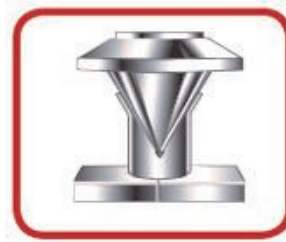
3 Rollers in Flaring Cone. Flare Formed above die block
