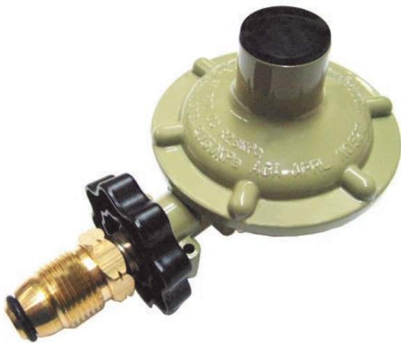
3/8 Female Single Stage POL Regulator with Hand Wheel. Capacity 125Mj/h
